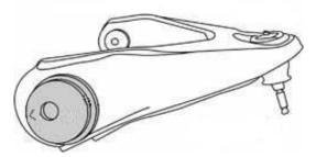
e) For **1999-2006** vehicles the distance between the two inner faces of the bushings should be 9 7/8". Make sure the bushings are centered in the arm.
