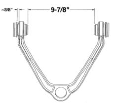
f) For **2007 up** vehicles the distance between the two inner faces of the bushings should be 9. Make sure the bushings are centered in the arm.
